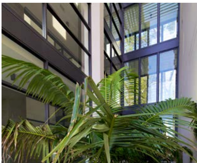
Figure 4L.9 Light wells can provide for daylight access to common areas. For habitable rooms of apartments, they should only be used as a secondary light source
