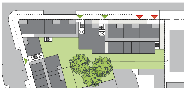
Figure 4M.6 Mixed use buildings may have a range of circulation spaces including multiple cores and gallery access
