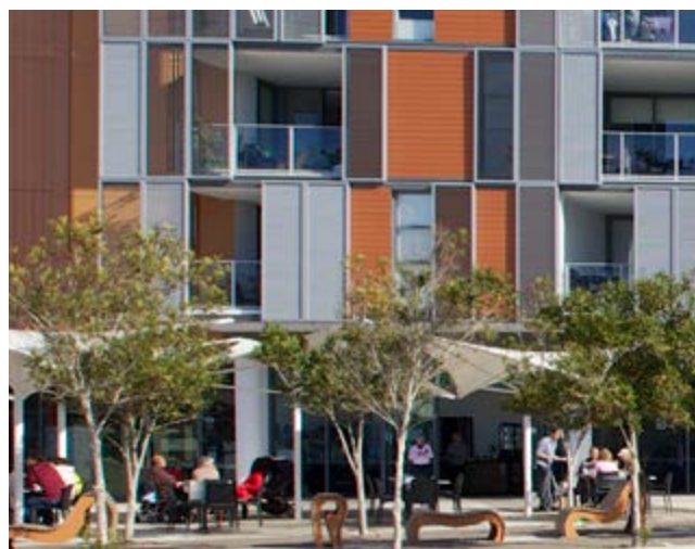
Figure 40.3 Ground floors often need to accommodate a range of uses such as retail, cafes and restaurants, and should provide increased ceiling heights to allow for maximum flexibility of use
