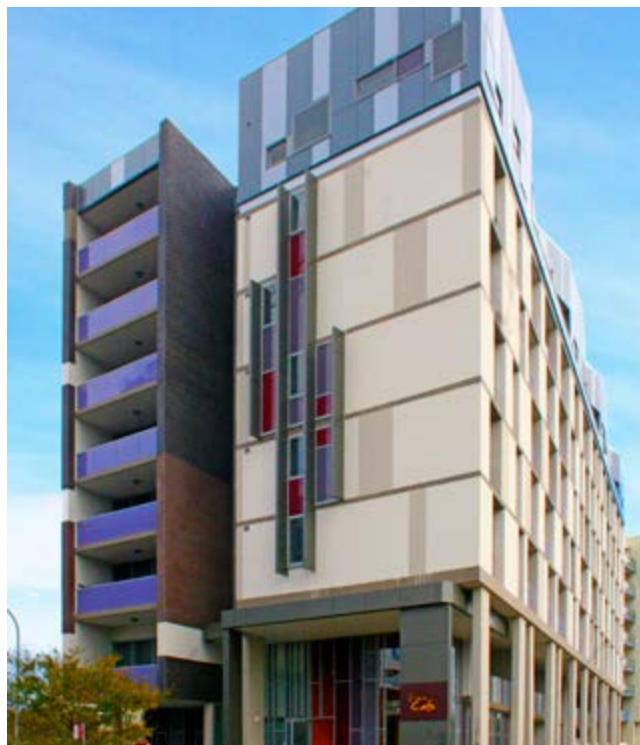
Figure 4C.1 Thoughtful modulation of the facade reduces the perceived depth and bulk of a building
