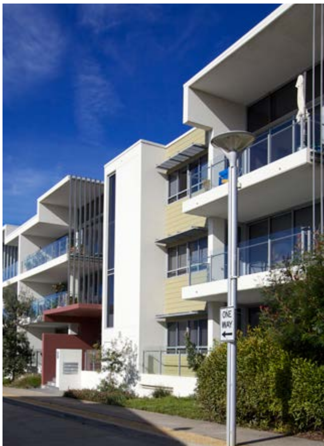
Figure 4X.3 Roof overhangs, hoods and drip lines protect walls from the elements (rain, sun, wind) reducing maintenance costs
