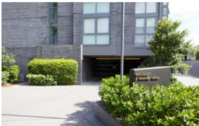
Figure 3H.3 The visual impact of vehicle entries can be minimised by an offset alignment of the driveway and screen planting
