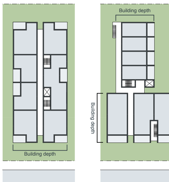
Figure 2E.2 These examples show how to measure building depth for different apartment building shapes
